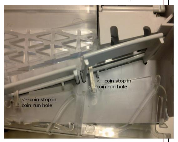
Then close the sort door, and replace the acceptor head back into the coin mech, ensure care is
