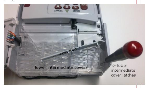
Remove the coin jam and replace the lower intermediate covers. Special care should be used to
